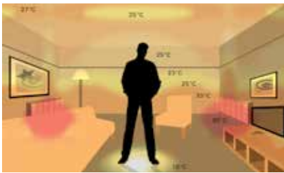
Heat radiation from a conventional heating system with radiators. Large temperature variations (18–65°C) in the room.
