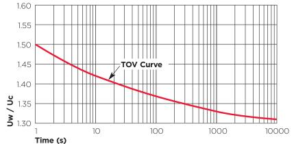
Temperature of samples (pre-heated): 60° C according to IEC 60099-4, Ed 2.0 2004. TOV Curve applies to an arrester which has a pre-stress applied prior to TOV verification. This pre-stress is equivalent to one high current impulse of 100kA, 4/10 as per the switching surge operating duty test.
