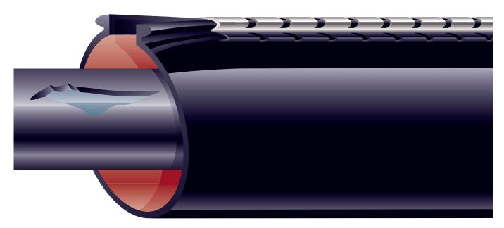
Labour-saving installation. Fitting and sealing all in one step. Abrasion and corrosion resistant. Each size covers a range of cable sizes. Raychem's distinctive closure system, which incorporates a stainless steel channel slid over rails on the sleeve, keeps the wraparound in place during installation but can be easily removed when the adhesive has set.
