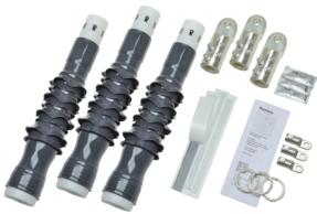
Raychem terminations CSTI/O cold shrink terminations are made from a high performance, liquid silicone material which is specially formulated for excellent tracking and split resistance. The extra-long, silicone stress cone is integrated within the termination which ensures correct positioning. Moisture sealing at the lug is integrated into the termination body, eliminating the need for additional sealing tapes.
