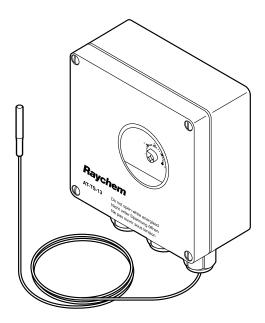
AT-TS thermostats provide temperature control in safe area. The temperature set point can be checked through a window in the lid. LED's are providing an indication when cables are energized (Heating ON) or when the temperature sensor is defect (sensor break or sensor short-circuit).
